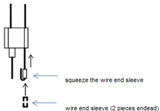
Push the wire end ferrules over the wire rope and allow the rope to protrude by approx. 7 mm. Now crimp the wire end sleeve firmly with a pair of combination pliers. Then fold over the protruding piece of rope and push it back into the hole of the stopper.
