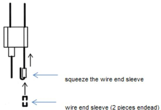
Push the wire end ferrules over the wire rope and allow the rope to protrude by approx. 7 mm. Now crimp the wire end sleeve firmly with a pair of combination pliers. Then fold over the protruding piece of rope and push it back into the hole of the stopper.
