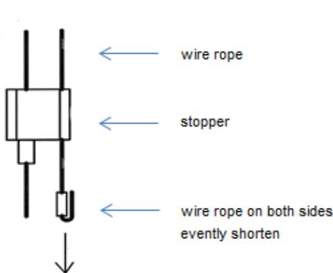
Pull the wire rope downwards out of the stopper and shorten it on both sides to the desired length.
